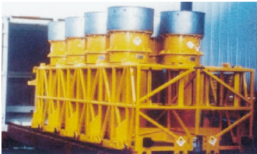
Figure 3: A plutonium shipment of 10 FS47 casks in vertical position in a rack, and its loading in an unarmoured truck, as commonly practiced in France
