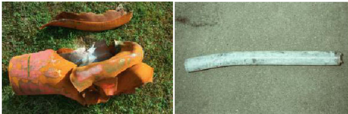
Figure 4: Example of the impact of an explosive device on the intermediate copper shell (left) and the inner container (right) of a FS47
